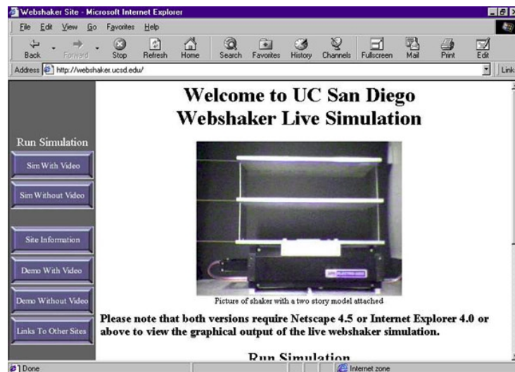
Figure 2. Webshaker Live Simulation. This experiment can be controlled and observed remotely (via teleoperation and teleobservation), in addition to analytically, via a Webservice at the University of California at San Diego ( http://webshaker.ucsd.edu ).
