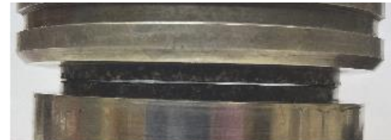
Pore space opens during sliding
