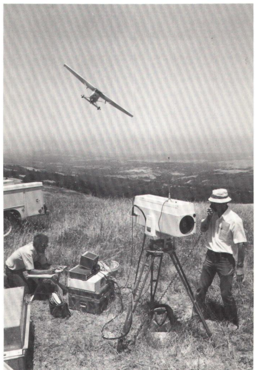
USGS survey team using a laser beam geodolite to monitor motion between fixed points on either side of the San Andreas fault. Aircraft gathers information on atmospheric conditions between geodolite and target several kilometers away.
